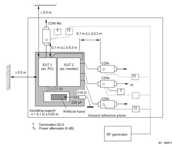
**Note:** 1.The EUT clearance from any metallic obstacles shall be at least 0,5 m.
